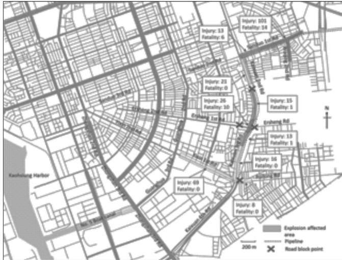
*Fig. 1. The explosion affected area, the distribution of casualties and the pipeline route*
